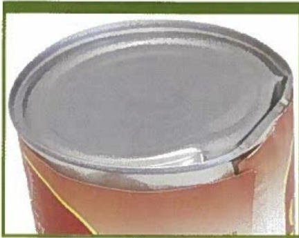
Severe dent in seam
